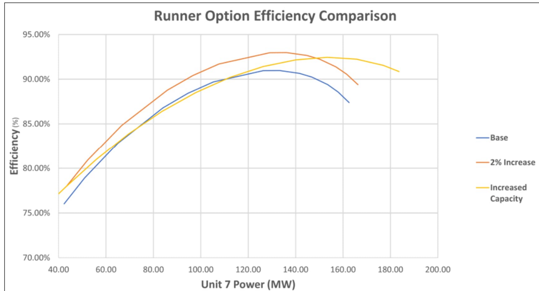
Figure 3-3: Efficiency Characteristics for the Various Runner Upgrade Options
